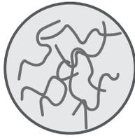
PVC and PETG are amorphous polymer materials which means their structure is made up of polymer chains which have no specific structure.
